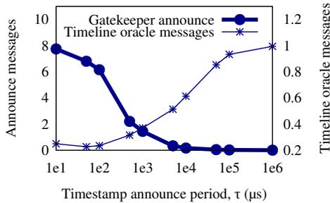
**Figure 14:** Coordination overhead, measured in terms of timestamp announce messages and timeline oracle calls, normalized by number of queries. High clock announce frequency results in large gatekeeper coordination overhead, whereas low frequency causes increased timeline oracle queries.
