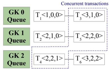
**Figure 6:** Each shard server maintains a queue of transactions per gatekeeper and executes the transaction with the lowest timestamp. When a group of transactions are concurrent (e.g.  $T_3$ ,  $T_4$ , and  $T_5$ ), the shard server consults the timeline oracle to order them.
