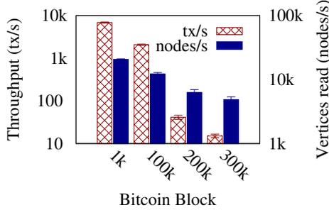
**Figure 8:** Throughput of Bitcoin block render queries in CoinGraph. Each query is a multi-hop node program. Throughput decreases as block size increases since higher blocks have more Bitcoin transactions (more nodes) per query.
