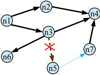
**Figure 1:** A graph undergoing an update which creates ( $n_5, n_7$ ) and deletes ( $n_3, n_5$ ) concurrently with a traversal starting at  $n_1$ . In absence of transactions, the query can return path ( $n_1, n_3, n_5, n_7$ ) which never existed.
