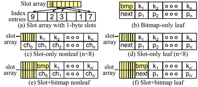
**Figure 8: wB<sup>+</sup>-Tree node structures. (For a slot+bitmap node, the lowest bit in the bitmap indicates whether the slot array is valid. Slot 0 records the number of valid entries in a node.)**
