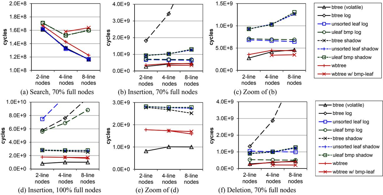
**Figure 11: Index performance on a cycle-accurate simulator modeling PCM-based NVMM. (We bulkload a tree with 20M entries, then perform 100K random back-to-back lookups, insertions, or deletions. Keys are 8-byte integers.)**
