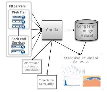
Figure 1: High level overview of the ODS monitoring and alerting system, showing Gorilla as a writethrough cache of the most recent 26 hours of time series data.
