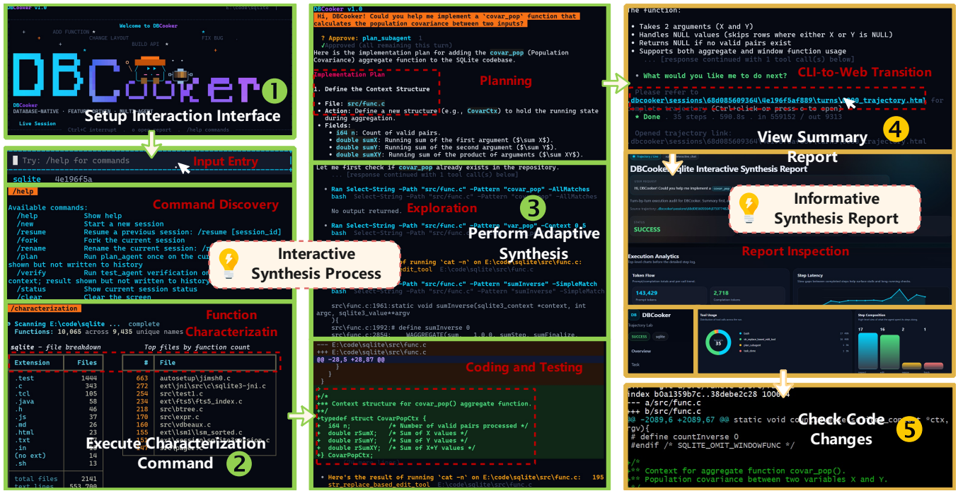
Figure 2: End-to-End Workflow of DBCooker (from the initial user CLI function request to the final web synthesis report).
