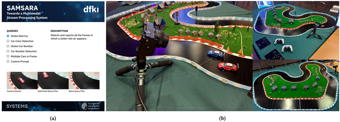
Figure 3: (a) Main UI for selecting queries targeting tasks such as color detection, OCR, and aggregation. (b) Camera setup for the simulated street monitoring scenario, where live video streams are processed using naive and Samsara-optimized queries.
