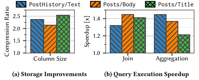
Figure 12: Compression ratio and join/aggregation speedup on the StackOverflow dataset in Umbra. We report the improvements relative to the baseline w/o tokenization.
