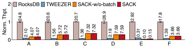
Figure 9: Exp#1 (Performance under YCSB core workloads). We plot the throughput normalized by RocksDB’s. We also report the absolute throughput in KOPS above each bar.
