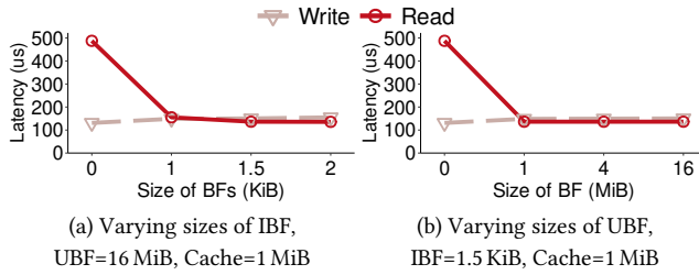
Figure 14: Exp#8 (Impact of the sizes of BFs). We vary the sizes of per-Ilog insert BFs (IBF) and update BF (UBF), while fixing the in-enclave LRU cache for per-Ilog insert BFs (Cache) as 1 MiB. A zero size means BFs are disabled.
