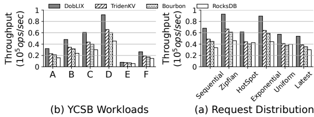
Figure 13: Throughput Comparison on YCSB macrobenchmarks and various distribution workloads.
