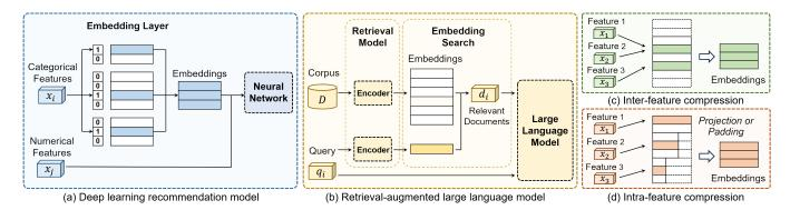
Figure 2: (a) A typical DLRM. (b) A typical retrieval-augmented LLM. (c) An example of inter-feature compression, the original 8 features now share 4 embeddings. (d) An example of intra-feature compression, each embedding is compressed individually.
