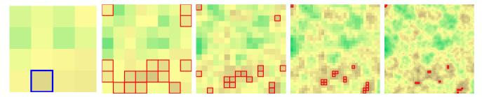
Figure 1: From left to right: five increasing resolutions of terrain height: 4x4, 8x8, 16x16, 32x32, 64x64. The blue square is the highest square in the lowest resolution. The red squares are the 16 highest squares in each subsequent resolution.
