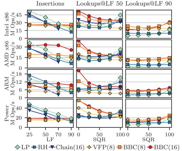
**Figure 8: Performance of BBC (8-bit and 16-bit fingerprints) and VFP (8-bit FPs), linear probing (AoS), robin hood (recalculating), and chained hashing (16-bit FP budget). We show the largest available register size.**
