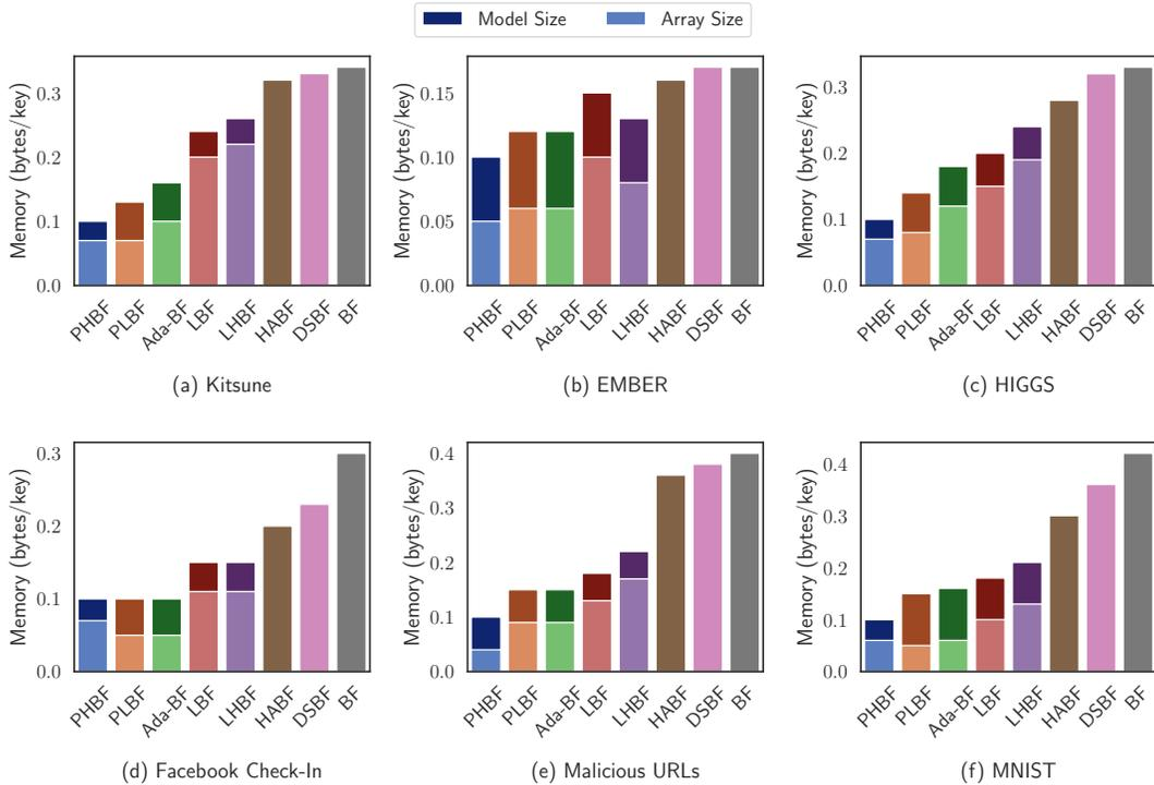
Figure 6: Comparison of bit array size and model size. The light (bottom) bar shows the bit array size and the dark (top) bar shows the model size. Note that some baselines do not use a model, and the size is entirely due to the bit array.
