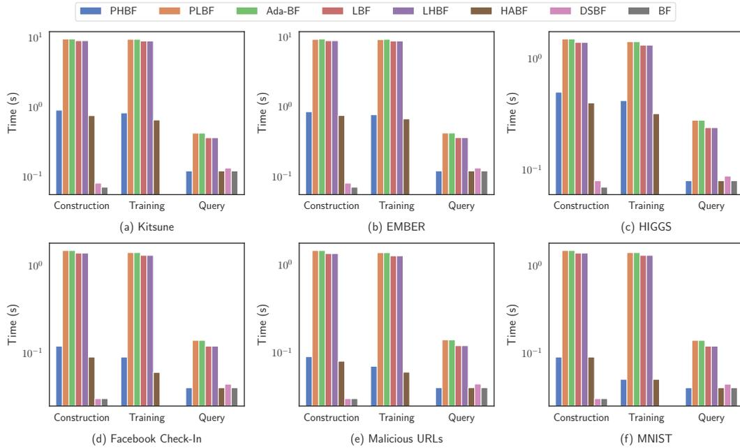
**Figure 7: Comparison of construction time and time per 1000 queries. The set of first 5 methods utilizes the sets  $X$  and  $Y$  to train a model, leading to higher construction time compared to the last two, which do not use them.**
