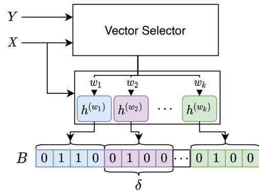
**Figure 2: Architecture of PHBF.** Given  $X$  and  $Y$ , Vector Selector selects  $k$  random vectors. These are used to compute the  $k$  hash functions, each populating their own partition of size  $\delta$  in  $B$ .
