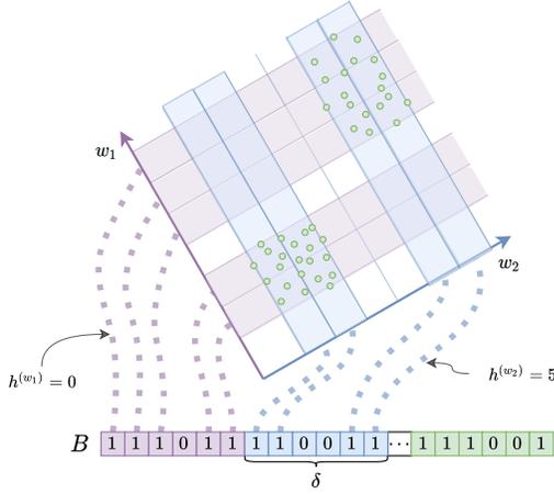
**Figure 3: Hash computation and Bit Array population.** The set  $X$  is represented by the green points. The figure shows 2 out of  $k$  random vectors.  $X$  is projected on to  $w_1$  and  $w_2$ . The range of the projection is divided into  $\delta$  bins, and the bins occupied by  $x \in X$  is set as 1 in  $B$ .
