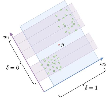
**Figure 4: Role of  $\delta$  in discriminating  $y \in Y$  from the points from  $X$ : The hash function  $h^{(w_2)}$  cannot separate  $y$  with  $\delta = 1$ , and generates a false positive. The hash function  $h^{(w_1)}$  with  $\delta = 6$  can successfully separate  $y$  from  $X$ .**
