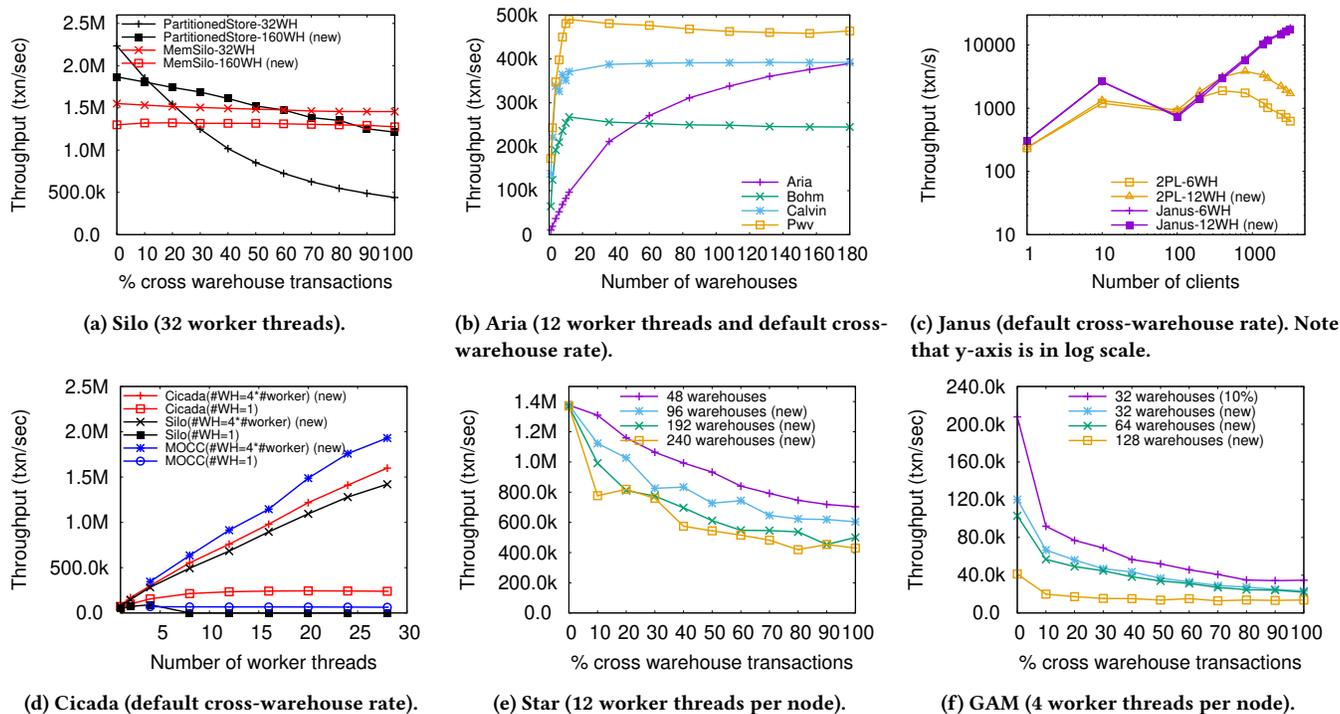
**Figure 1: Changing the number of warehouses, the percentage of cross warehouse transactions, and the number of workers/clients for different systems. Lines with (new) tags are those not existed in the original articles.**
