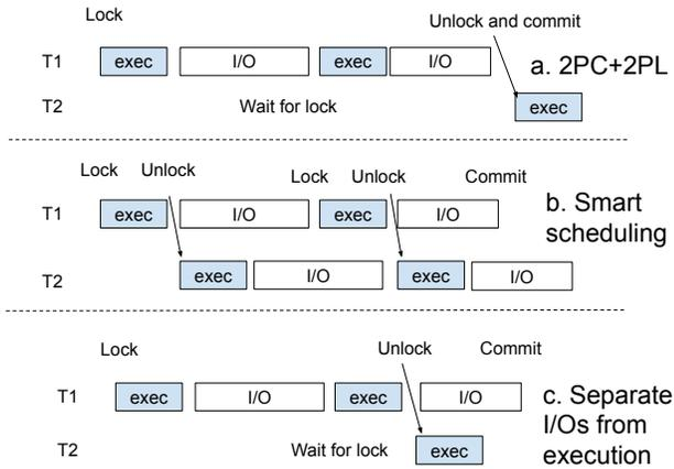
Figure 2: Reducing I/Os during a critical section.
