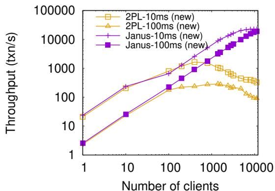
Figure 3: Throughputs of Janus and 2PL with extra network latencies (6 warehouses and default cross-warehouse rate). Note that y-axis is in log scale. Lines with (new) tags are those not existed in the original articles.
