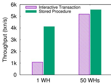
Figure 4: TPC-C throughputs of H2 with interactive transactions and stored procedures (WH=Warehouses).
