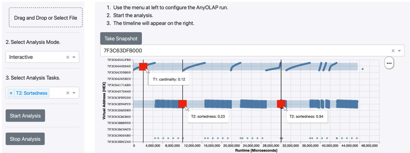
**Figure 5: The GUI and the timeline of an AnyOLAP run. All intercepted memory allocations, their lifetime, as well as all taken snapshots are visualized. Further, the executed analysis functions are shown. Hovering the snapshot reveals the result. (Multiple visualizations have been merged to show the result of all executed tasks in one figure.)**
