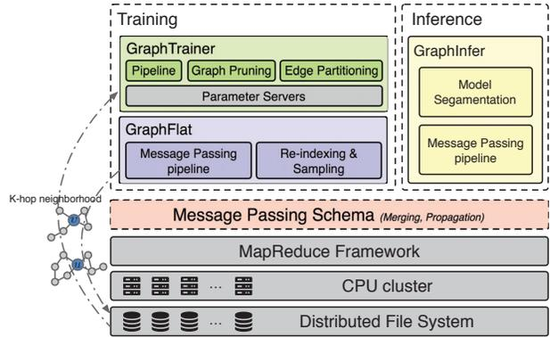
Figure 1: System architecture of AGL.
