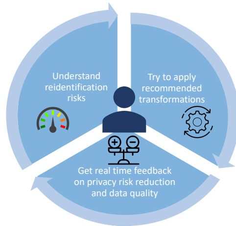
Figure 1: Depiction of the X^2R^2 data anonymization process with the human-in-the-loop. The tool explains the reidentification risks currently existing in the data and recommends a set of the best data transformation operations. The user can try out the different recommended data transformations and monitor their effects on the trade-off between reidentification risk and data quality.
