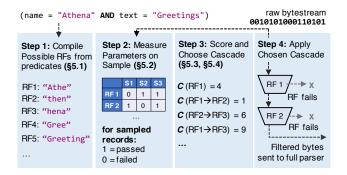
**Figure 2:** An overview of Sparser. Sparser builds a cascade of raw filters to filter data before parsing it.
