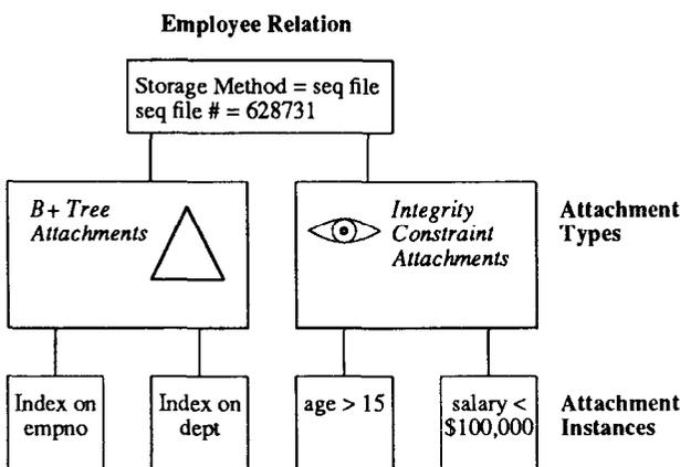
Figure 1: Storage Method and Attachment Example.
