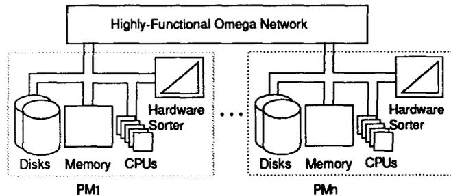
Figure 1: Architecture of Super Database Computer
