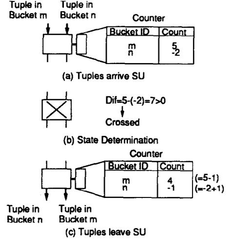
Figure 11: State Determination in Switching Unit
