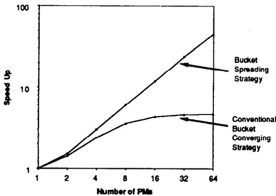
Figure 18: Comparison of Speed Up (2)
