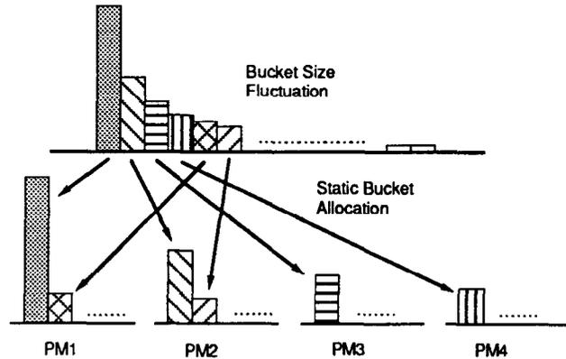
Figure 3: Load Unbalancing Caused by Data Skew
