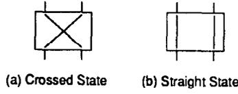
Figure 10: Two States of Switching Unit
