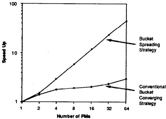
Figure 17: Comparison of Speed Up (1)
