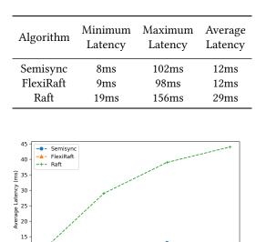
Figure 4. Effect on latency with increasing replica set size
