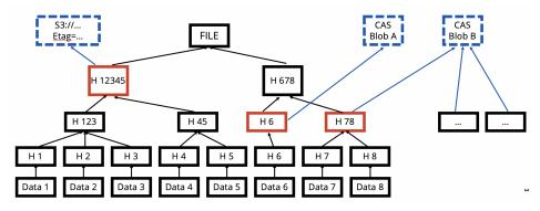
Figure 3: To reconstruct a given file, the Merkle Tree is traversed to find data sources to concatenate. The solid red nodes indicate the set of nodes which are sub-ranges in other storage sources (dashed blue nodes). H12345 can be read from an existing S3 object, H6 can be directly queried from the CAS, and H78 is a sub-range in another CAS entry (Blob B).
