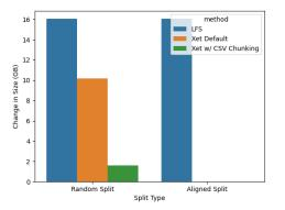
Figure 5: Incremental storage cost of adding a branch with a dataset split. In the *random split*, the rows are randomly shuffled into two files. In the *aligned split*, the file is simply partitioned. LFS required complete storage of 16GB. Xet dedupes the random split to 11GB, and 185KB for the aligned split. Xet+CSV requires 1.6GB for the random split and 173KB for the aligned split. Aligned split bars are too small to display See Sec. 6.4 for details.
