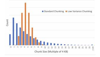
Figure 2: Example chunk size distribution using a standard rolling hash chunking procedure, vs the low variance chunking procedure on 4.3GB of compressed CentOS disk images. We observe the low variance chunking procedure is more Gaussian distributed and avoids both excessively small and large chunks.
