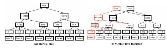
Figure 1: (a) Content Defined Merkle Tree. Each leaf chunk is derived from a Content Defined Chunking procedure. Nodes are merged using a simple hashing rule: a partition is inserted whenever the hash modulo a target child count equals 0 with constraints on a minimum / maximum child count. (b) Insertion of a new chunk (Data 0) can maintain tree stability. New nodes are in red.
