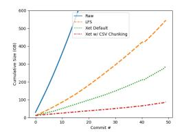
Figure 4: Cumulative storage cost for committing 50 CORD-19 dataset versions from 2021-02-01 to 2022-06-02. The Y axis is truncated for readability. LFS required 545GB, Xet required 287GB including a 2.4GB MerkleTree. Xet+CSV required 87GB including a 1.7GB MerkleTree. See Sec. 6.4 for details.
