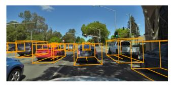
Figure 1: AV camera image with vehicle bounding-boxes [40]
