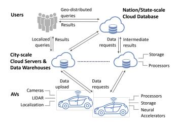
Figure 2: AV query system architecture
