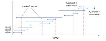
Figure 4: Visualizing objects entering and leaving an AV's view. Dashed lines represent frames chosen by the *min-frame* algorithm.
