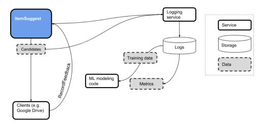
Figure 2: Architecture of ItemSuggest's integration with machine-learning workflow.
