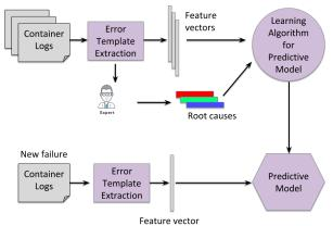
Figure 3: Approach for automatic root cause analysis (RCA)
