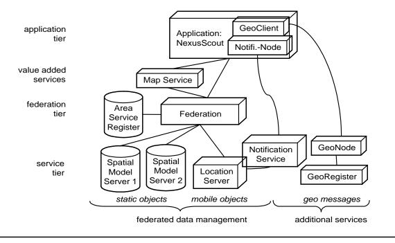
Figure 2: Architecture of Demonstrated Nexus Platform
