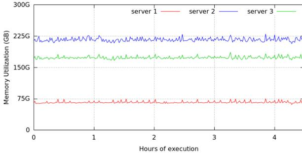
Figure 9: Memory utilization of servers ingesting data in real time with rollup enabled.
