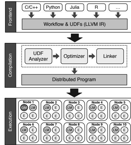
**Figure 1: An overview of our proposed architecture.** The *Frontend* allows users to compose UDF workflows in any LLVM-supported language (top boxes). These workflows are then translated to self-contained distributed programs during the three-stage *Compilation* process. Finally, the *Execution* phase deploys the distributed programs on a cluster, shown as 10 nodes (labeled boxes) each with four cores (circles inside the boxes) that have specialized execution roles (GM, LM, E).
