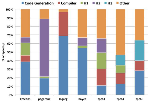
**Figure 3: A performance breakdown with percentage speedups achieved by TUPLEWARE over Spark from Section 7.2.**
