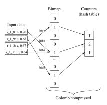
Figure 4: BFHM bucket structure
