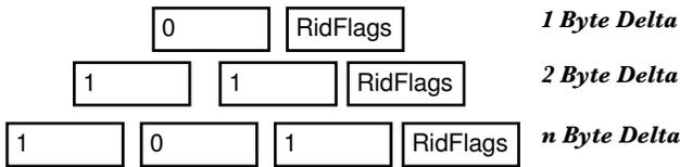
**Figure 7: Delta encoding to support forward & reverse scans**
