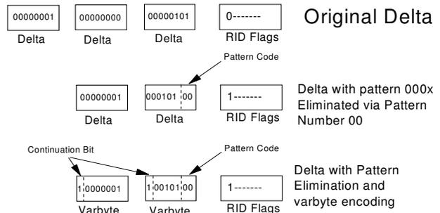
**Figure 8: Delta encoding with pattern elimination**
