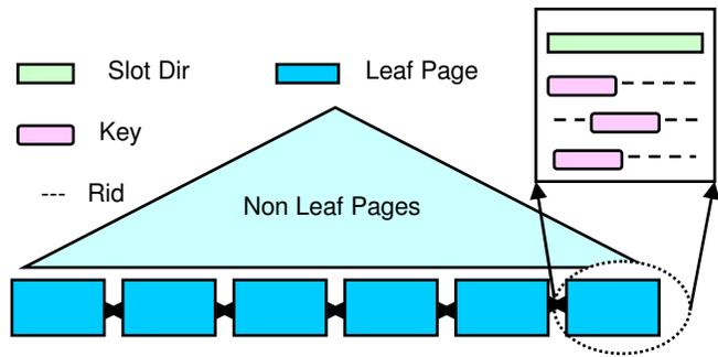
**Figure 2: Structure of a B+ Tree in DB2**
