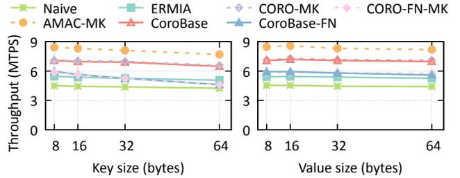
**Figure 10: Throughput of read-only YCSB (10 reads per transaction) under varying key/value sizes and 96 hyperthreads.**
