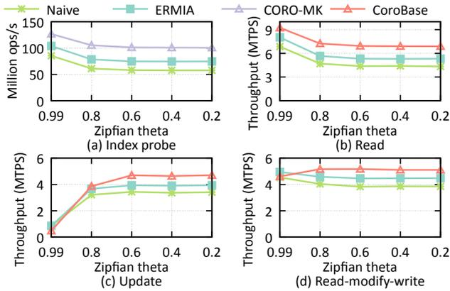
Figure 12: YCSB throughput with 96 hyperthreads and varying skewness (larger theta indicates more skewed access).
