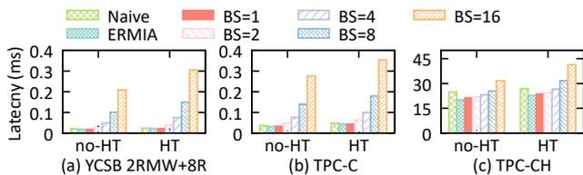
**Figure 16: Average transaction latency under varying batch sizes (BS=1–16) with asynchronous commit. The end-to-end impact is expected to be small with group/pipelined commit.**
