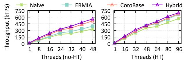
Figure 14: Throughput of the read-only TPC-CR workload.
