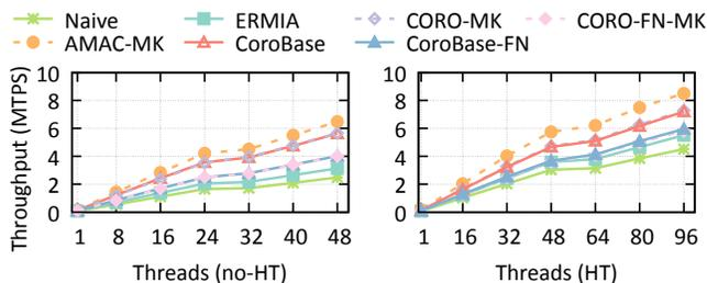
**Figure 6: Throughput of a read-only YCSB workload (10 reads per transaction) without (left) and with (right) hyperthreading. CoroBase matches the performance of multi-key variants but without requiring application changes.**
