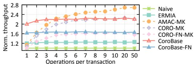
**Figure 7: YCSB read-only performance normalized to Naïve under 48 threads. CoroBase also benefits very short transactions (1–4 operations) while multi-key based approaches inherently cannot under thread-to-transaction.**
