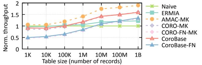
**Figure 11: YCSB read-only (10 reads per transaction) performance normalized to Naïve under 96 hyperthreads and varying table sizes.**
