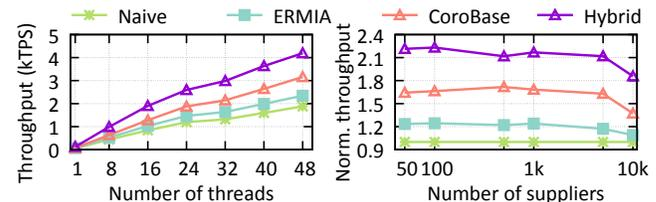
Figure 15: TPC-CH scalability (left) and throughput with 48 threads normalized to Naïve (right). CoroBase reaps more benefits from prefetching with more read operations.
