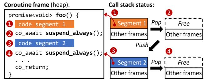
Figure 2: Stackless coroutine that directly uses the underlying thread’s stack. States (e.g., local variables and return value) are maintained in dynamically allocated memory.
