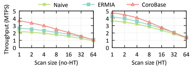
**Figure 9: Throughput of a YCSB scan workload. The benefits of prefetching diminish with larger scan sizes: more records can be directly retrieved in leaf nodes using B-link-tree structures.**
