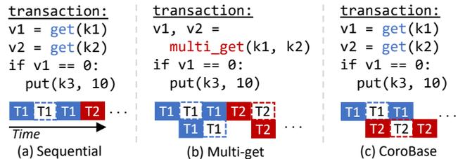
Figure 1: Data access interfaces and execution under (a) sequential execution (no interleaving), (b) prior approaches that require multi-key interfaces, (c) CoroBase which hides data stalls and maintains backward compatibility.
