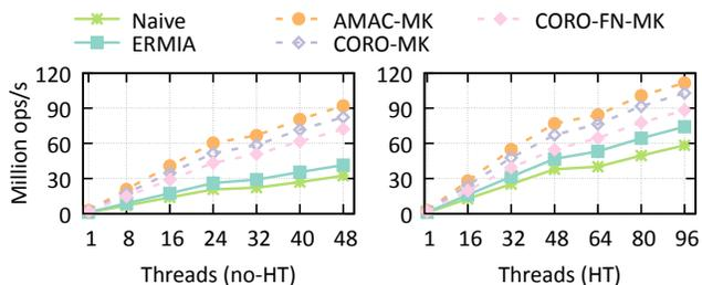
**Figure 5: Index probing throughput with hyperthreading disabled (left) and enabled (right). Fully-nested coroutines are ~30% slower than AMAC. Flattened coroutines (CORO-MK) reduce the gap to 8–10% under high concurrency.**
