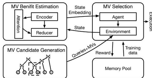
Figure 9: Encoder-Reducer Based View Recommender
