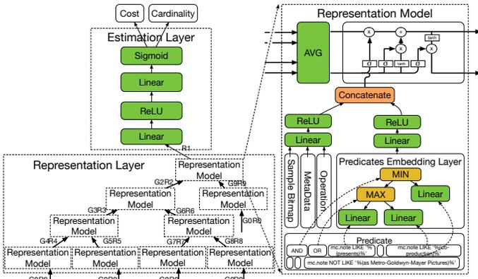
Figure 3: Tree-LSTM Based Cost Estimator
