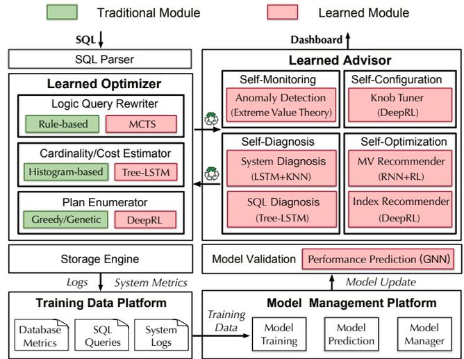
Figure 1: The openGauss Architecture
