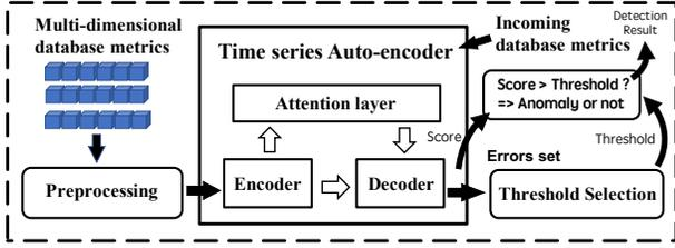
Figure 5: LSTM-Based Anomaly Detection
