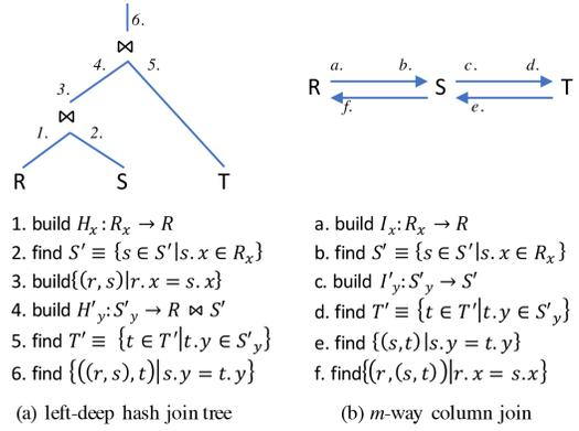
Figure 5: Left-deep hash join vs.  $m$ -way column join.
