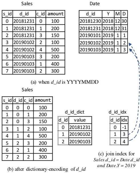
Figure 4: Dictionary-based join index.
