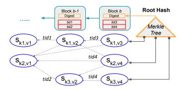
Figure 5: A Merkle DAG for storing provenance.  $s_{k_2,v_4}$  and  $s_{k_3,v_4}$  updated by the same transaction  $(tid_4)$ , but their dependencies are different. b contains two transactions,  $tid_3$  and  $tid_4$ . Its latest states include  $s_{k_1,v_3}$ ,  $s_{k_2,v_4}$ ,  $s_{k_3,v_4}$ , from which a Merkle tree is built.
