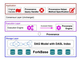
Figure 9: *LineageChain's* software stack. The original storage layer is replaced with the implementation that supports fine-grained provenance. The original execution layer is instrumented with a provenance capture engine. The application layer contains the new helper method and provenance query APIs. The consensus layer is unchanged.
