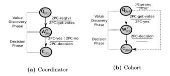
Figure 1: State machine representation of 2PC.
