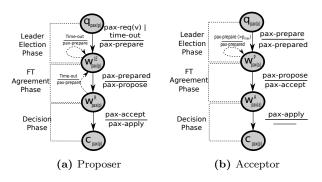
Figure 2: State machine representation of Paxos.
