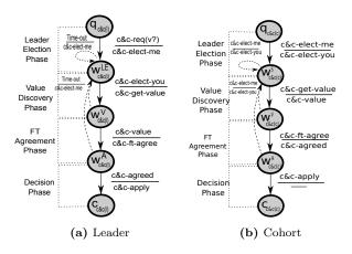
Figure 4: State machines of the C&C framework.
