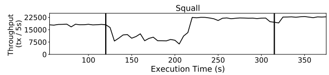
Figure 2: With TPC-C workload, Squal [12] renders a drop in throughput in the binning of the migration period.
