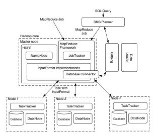
Figure 1: The HadoopDB System Architecture [18]
