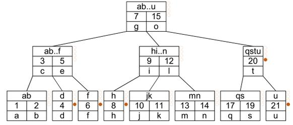
**Figure 1:** Classic B-tree augmented with aggregates (top cell of each node). The notation for stored aggregates omits  $\otimes$ , e.g.,  $qstu$  is shorthand for the value of  $q \otimes s \otimes t \otimes u$ .
