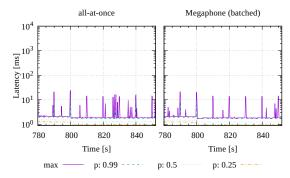
Figure 11: NEXMark query latency for Q7,  $4 \times 10^6$  requests per second, reconfiguration at  $800 \, \text{s}$ .
