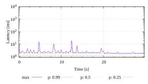
Figure 5: NEXMark query latency for Q1,  $4 \times 10^6$  requests per second, reconfiguration at 10 s and 20 s. No latency spike occurs during migration as the query does not accumulate state.
