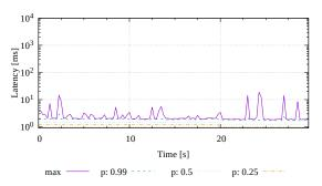
Figure 6: NEXMark query latency for Q2,  $4\times10^6$  requests per second, reconfiguration at  $10\,\mathrm{s}$  and  $20\,\mathrm{s}$ . No latency spike occurs during migration as the query does not accumulate state.
