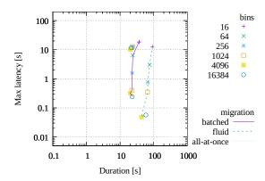
Figure 16: Key-count migration latency vs. duration, varying bin count for a fixed domain of  $4096 \times 10^6$  keys. The vertical lines indicate that increasing the granularity of migration can reduce maximum latency for fluid and batched migrations without increasing the duration. The all-at-once migration datapoints remain in a cluster independent of the migration granularity.
