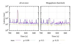
Figure 10: NEXMark query latency for Q6,  $4 \times 10^6$  requests per second, reconfiguration at  $800 \, \text{s}$ .
