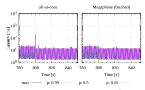
Figure 9: NEXMark query latency for Q5,  $4 \times 10^6$  requests per second, reconfiguration at 800 s with time dilation.
