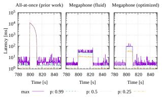
Figure 1: A comparison of service latencies in prior coarse-grained migration strategies (all-at-once) with two of Megaphone's fine-grained migration strategies (fluid and optimized), for a workload that migrates one billion keys consisting of 8 GiB of data.
