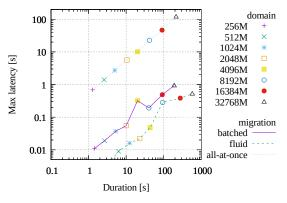
Figure 17: Key-count migration latency vs. duration, varying domain for a fixed rate of  $4 \times 10^6$ . As the domain size increases the migration granularity increases, and the duration and maximum latencies increase proportionally.
