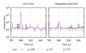
Figure 8: NEXMark query latency for Q4,  $4 \times 10^6$  requests per second, reconfiguration at  $800 \, \mathrm{s}$ .
