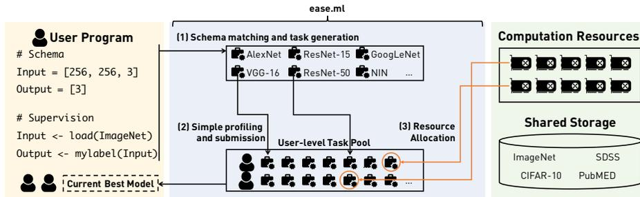
Figure 2: System architecture of `ease.ml`.
