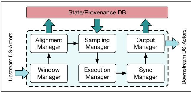
**Figure 3: A DataStorm-FE actor (DS-actor), with individual sub-modules.**
