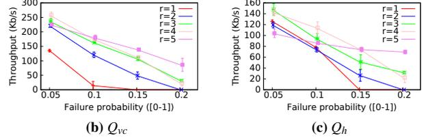
Figure 12: Throughput vs. node failures for replication  $r$
