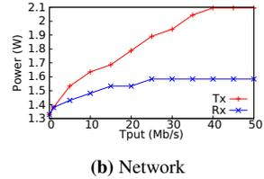
Figure 19: Power consumption on Raspberry Pi 3 Model B
