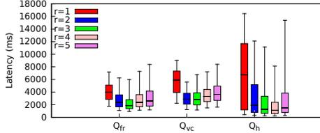
Figure 13: Latency with varying replication factor  $r$  (Roofnet) (Datapoints show 5/25/50/75/95<sup>th</sup> percentiles.)
