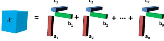
**Figure 1:** Illustration of an  $R$ -component CP model for a third order tensor
