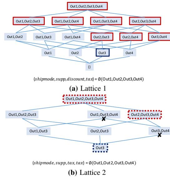
**Figure 3:** Optimizations in group-by discovery. (a) Group-by candidate nodes in Lattice 1 that are outlined in red are pruned by containment checking while the node outlined in black is pruned by keyness checking. (b) Lattice nodes that are needed for containment checking in Lattice 2 where the dotted nodes are propagated by the failure nodes in Lattice 1 and the crossed out nodes are pruned by overlapped mapping columns.
