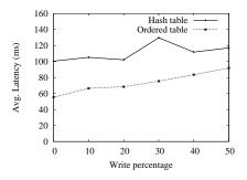
Figure 4: Impact of varying read:write ratio on the average request latency.
