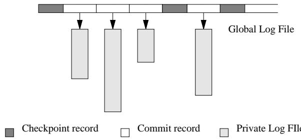
**Fig. 3.** The physical structure of the EOS log file
