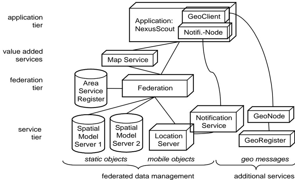
**Figure 2:** Architecture of Demonstrated Nexus Platform
