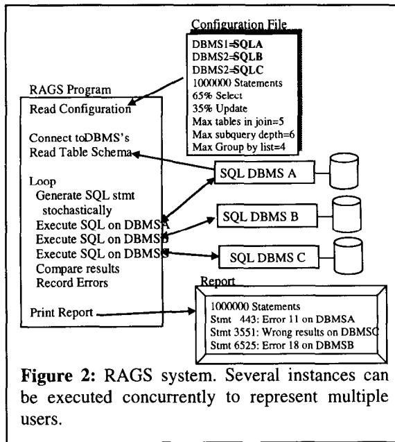
**Figure 2:** RAGS system. Several instances can be executed concurrently to represent multiple users.
