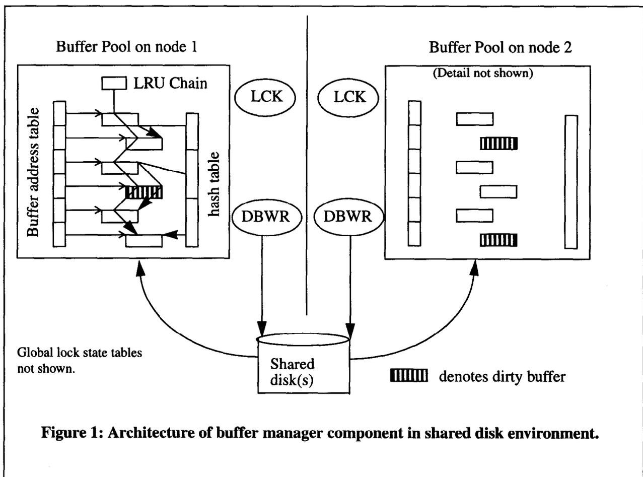
**Figure 1: Architecture of buffer manager component in shared disk environment.**
