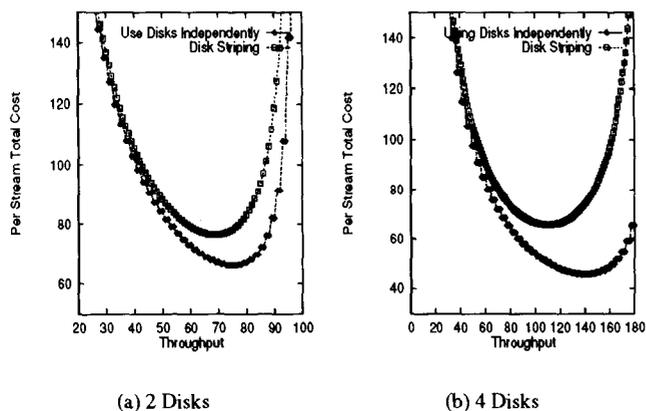
Figure 9: Per Stream Cost With Multiple Disks
