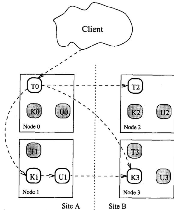
Figure 2: Processes involved in a simple transaction.
